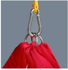
When rescuing with lifting gear, attention must be paid that **BOTH** rings of the belt system are hooked in. **(Picture 6)**
